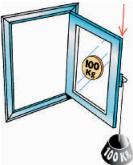
A supplementary load of 100 Kg is added for 5 minutes to the normal weight of the casement (100 Kg).
